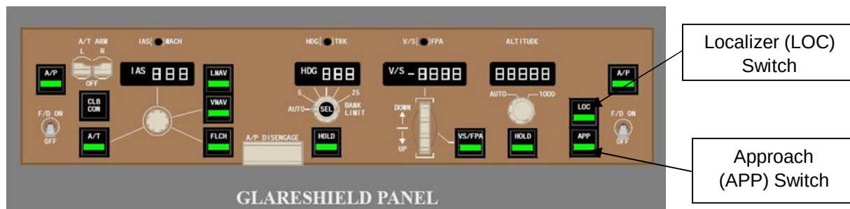
Figure 1.6ED Approach Mode Switches
