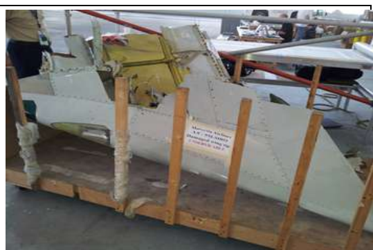
Figure 1.6B – Damaged Wing Tip
