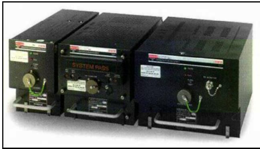
Figure 1.9M RFU (left), SDU (centre) and HPA (right)
